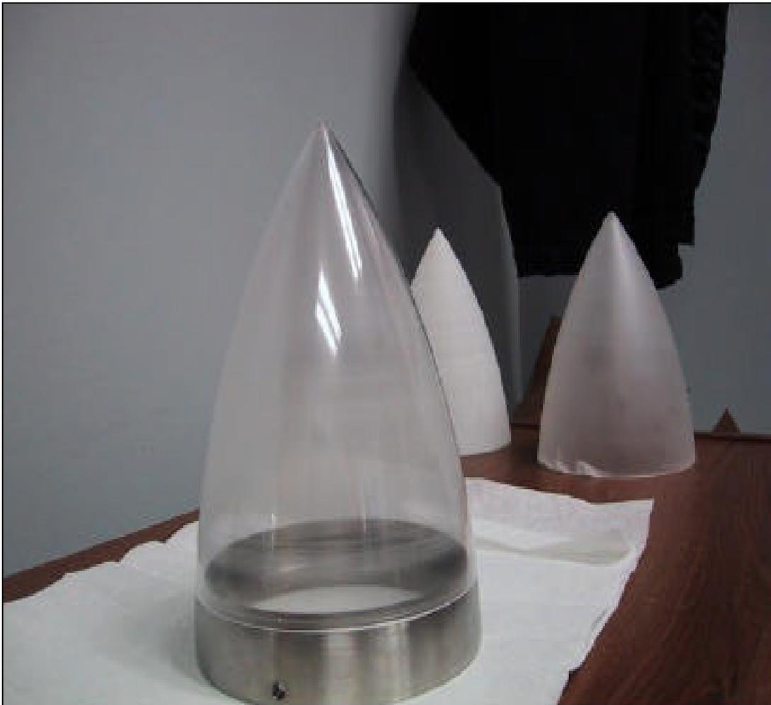
Figure 7: Finished ALON dome on mounting fixture.
