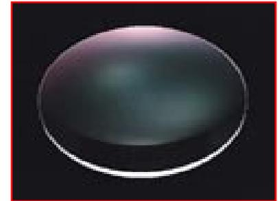
**Objective:** To quantify surface finish and form results obtainable on CaF<sub>2</sub> using the Nanotech 250UPL.
