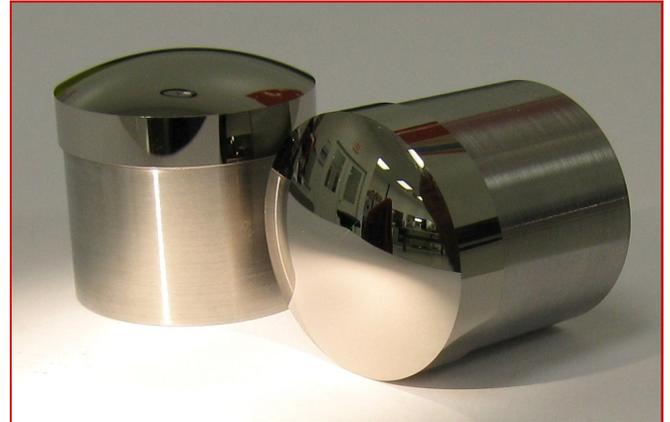
**Objective:** To quantify “champion” surface finish and form accuracy obtainable in electroless nickel plating using the Nanotech 250UPL.
