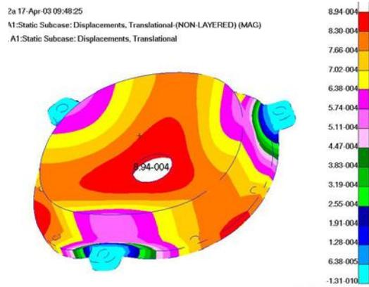
Fig. 2 Surface deformation diagram under 50g axial inertial load
