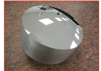
**Objective:** To quantify surface finish and form results obtainable on Aluminum using the Nanotech 250UPL.
