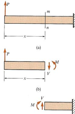
It is convenient to reduce the resultant to a shear force,  $V$ , and a bending moment,  $M$ . Because shear forces and bending moments are the resultants of stresses distributed over the cross section, they are known as **stress resultants** and in statically determinate beams can be calculated from the equations of static equilibrium.
