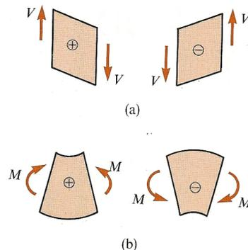
Positive shear forces always deform right hand face downward with respect to the left hand face. Positive bending moments always elongate the lower section of the beam.
