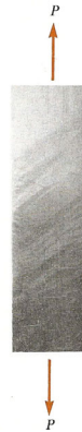
Fig. 2-32 Slip bands (or Lüders' bands) in a polished steel specimen subjected to axial tension
