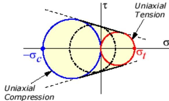
The **left circle** is for uniaxial compression at the limiting compression stress  $\sigma_c$  of the material. Likewise, the **right circle** is for uniaxial tension at the limiting tension stress  $\sigma_t$ .
