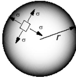
For reasons of symmetry, all the normal stresses on a small stress element in the wall must be identical. Furthermore, there can be no shear stress. The normal stresses  $\sigma$  can be related to the pressure  $p$  by inspecting a free body diagram of the pressure vessel. To simplify the analysis, we cut the vessel in half as illustrated.
