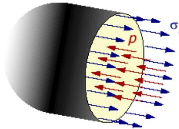
Summing forces in the longitudinal direction we obtain the same result as with the spherical pressure vessel.
