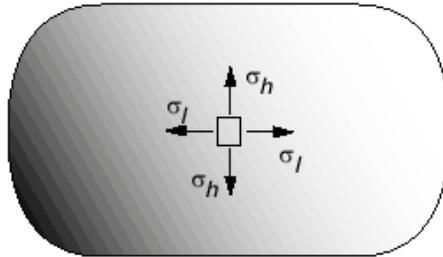
The coordinates used to describe the cylindrical vessel can take advantage of its axial symmetry. It is natural to align one coordinate along the axis of the vessel (*i.e. in the longitudinal or axial direction*). To analyze the stress state in the vessel wall, a second coordinate is then aligned along the hoop direction (*i.e. tangential or circumferential direction*).
