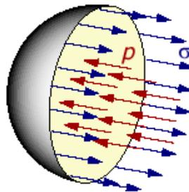
Since the vessel is under static equilibrium, it must satisfy Newton's first law of motion. In other words, the stress around the wall must have a net resultant to balance the internal pressure across the cross-section. Summing forces we obtain:
