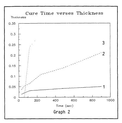
not measureable until 120 seconds of exposure at which time it was close to 250 mils. It appears that the cure was occurring uniformly throughout the film on initial exposure but was not sufficient to fully polymerize the material until a certain minimum exposure had occurred.
