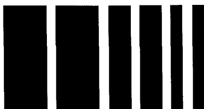
(a) Test bar code with alternating light and dark periods with decreasing bar width and spacing
