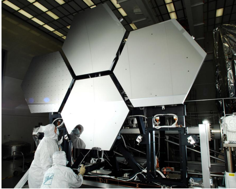
Figure 10. Assembly of JWST primary mirror segments at Marshall Space Flight Center
