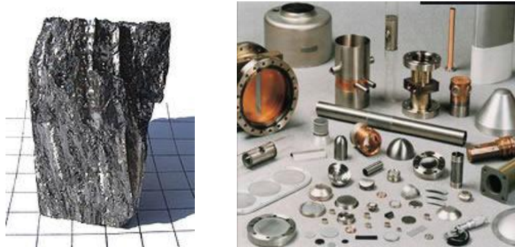
Figure 1. Beryllium – raw and machined
