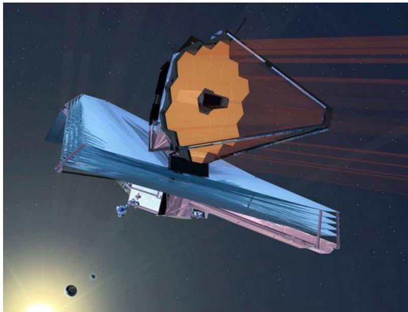
Figure 11. Concept drawing for James Webb Space Telescope showing primary and secondary mirrors
