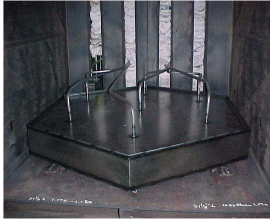
Figure 4. HIP can for hexagonal blank
