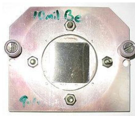
Figure 8. Beryllium window between a vacuum chamber and an x-ray microscope
