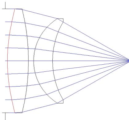
**Figure 1 - 2 element  $f/1$  transmission sphere**
