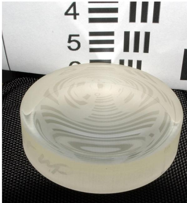
Figure 8 - Aspheric surface with 950 microns departure over 45 mm
