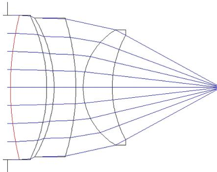
**Figure 2 – Three element f/1 transmission sphere example**
