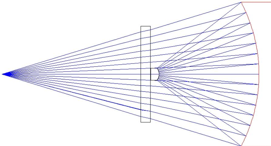
**Figure 3 - Null testing concave ellipse at conic foci**
