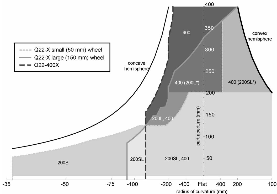
Figure 10 - Size capabilities of QED MRF machines (courtesy of QED)
