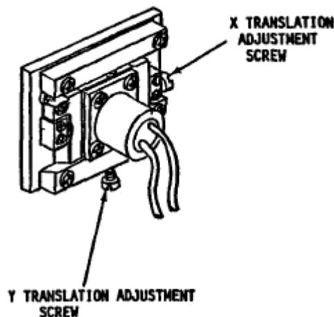
**Figure 2: Visible and star sense detector adjustment mechanism (Horchem & Korman, 1989)**
