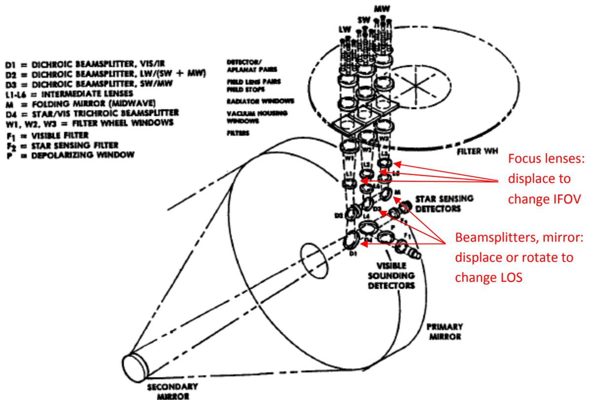
Figure 1: Schematic layout of optical system (Horchem & Korman, 1989)
