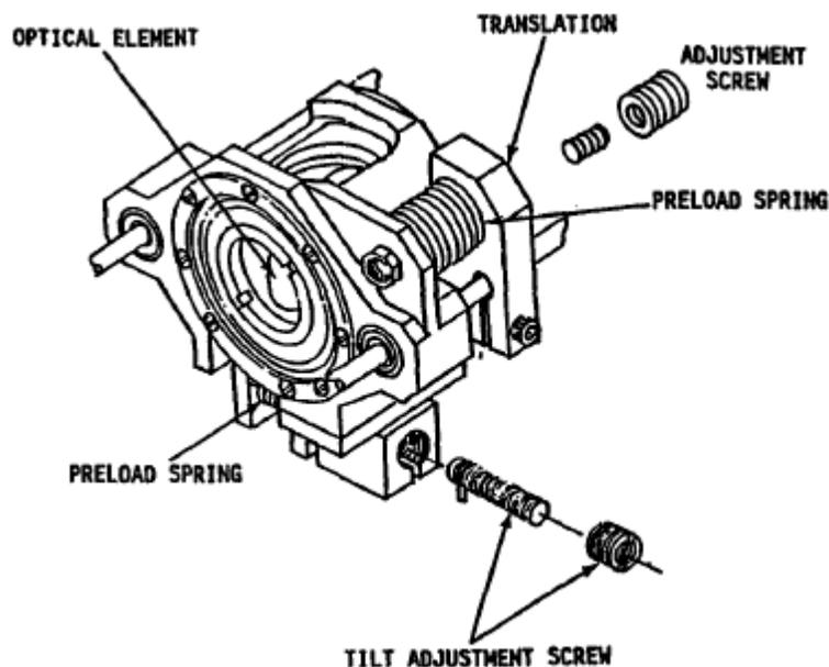
**Figure 3: Visible Mirror / beamsplitter adjustment mechanism (Horchem & Korman, 1989)**
