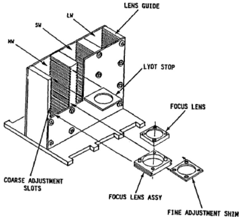
**Figure 4: Focus lens adjustment mechanism (Horchem & Korman, 1989)**
