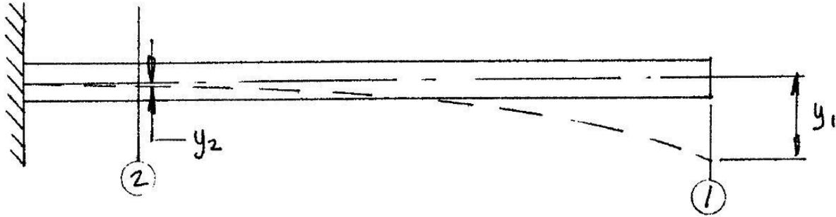
Figure 1: Vertical displacements along an elastic cantilever beam [1]
