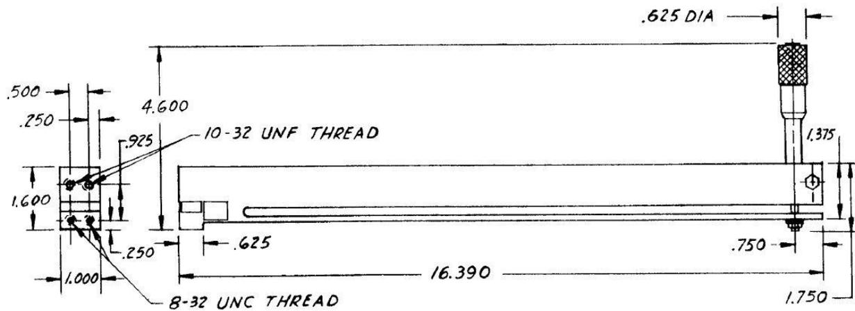
Figure 2: 6061-T6 actuator with one micron range and one angstrom resolution [1]
