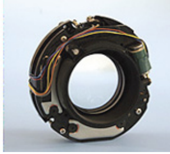
Figure 5: Nikon VR lens element and voice coil actuators
