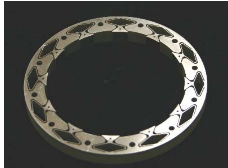
The diamond flexure lens cell design and manufactured titanium lens cell hub
