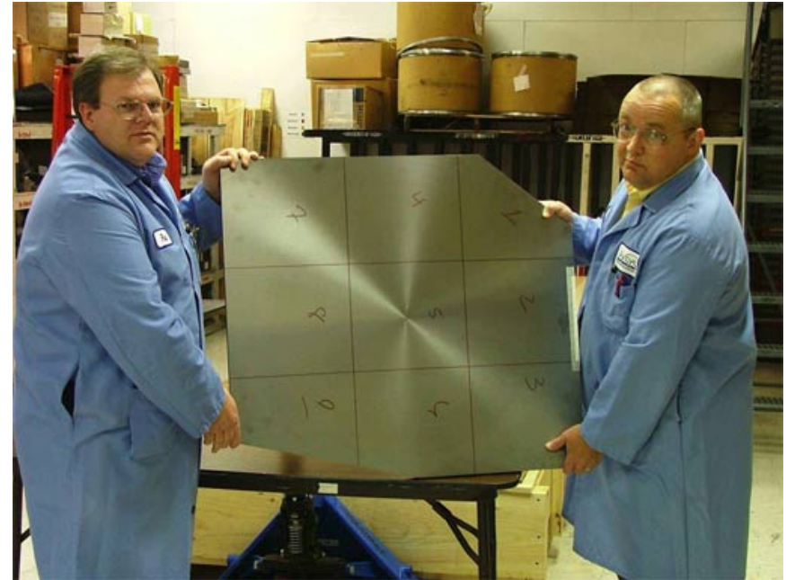
I-220H Heat Treated and Machined to Rough Shape
