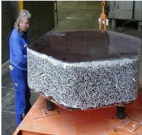
Figure 3: Raw Zerodur boule (left)
