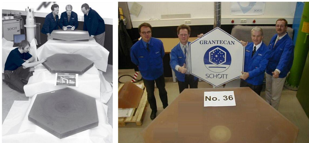
Figure 2 : Zerodur mirror blanks for LAMOST (left) and GTC (right)
