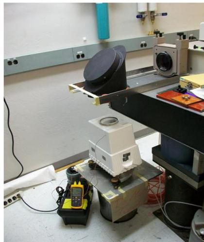
**Figure 5: Device configuration. It consists of a Fizeau interferometer, a fold mirror, a temperature chamber and a thermometer**
