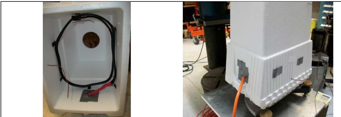
Figure 8: The pipe heater in the temperature chamber
