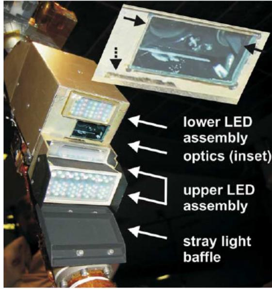
Figure 2: Engineering model of the RAC mounted to the Robotic Arm.
