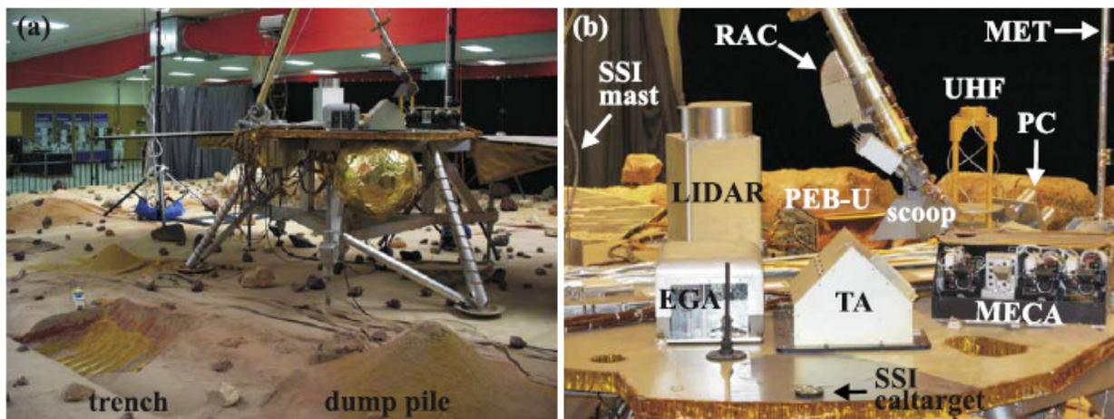
Figure 1: The engineering model of the Phoenix Lander located at a testing center in Tucson (a) and the RAC surrounded by other instruments of the lander (b).
