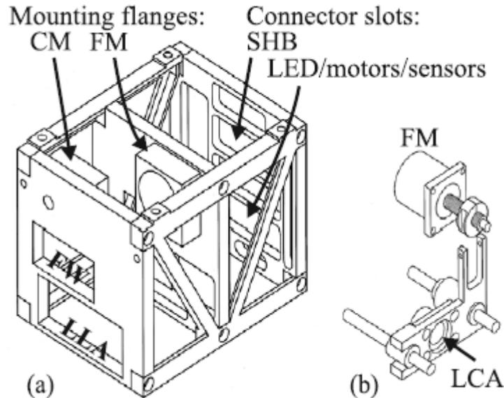
Figure 3: Optomechanical layout of the RAC. (a) The RAC frame and optical bench, including mounting slots for the front window (FW) and lower lamp assembly (LLA). The frame houses the CCD, cover motor (CM), focus motor (FM), and lens cell assembly (LCA). (b) The focusing mechanism.
