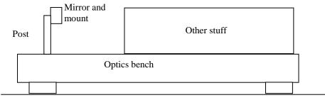
The mirror is mounted on a 20 cm long, 15 mm diameter steel post
