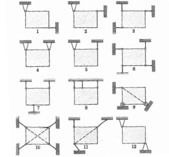
**2)** Each of these structures is staticly indeterminate: overconstrained.
