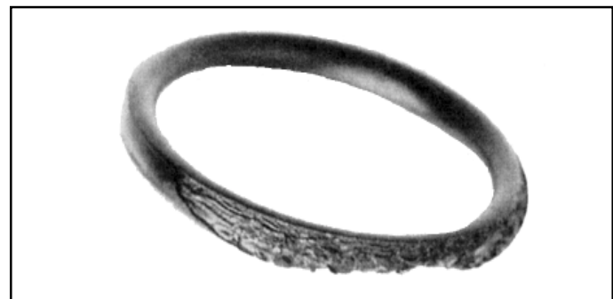
Figure 10-3: "Nibbled" Extruded O-Ring
