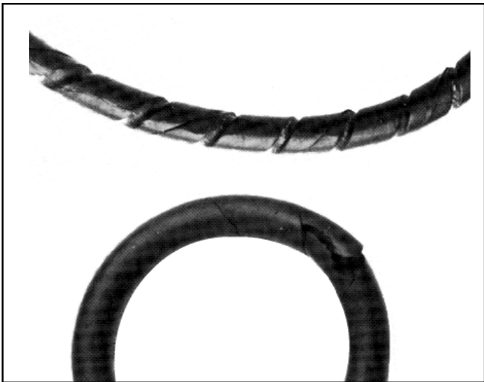
Figure 10-4: Twisted O-ring with spiral marking, or with spiral cuts in surface
