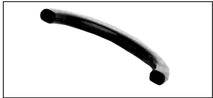
Figure 10-1: Characteristic compression set — high deformation
