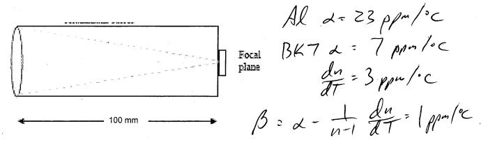
For 20°C temperature change, determine the change in focus in mm.
