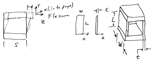
Provide the equations that would be used to determine  $k_x$  and  $k_y$ , the stiffness of the mechanism against forces in **each of the two directions** perpendicular to the motion allowed by the flexures.
