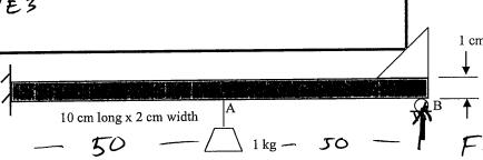
EI= TEB A 1 kg weight is attached at point A in the middle of the beam, causing it to distort.
