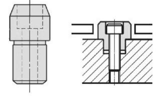
The Clearance Hole with the C-Bore feature lets you install the pin using S.H.C.S. when you have limited access to the back or side of the mounting plate. The disadvantage if this pin is its size. This design can not be used when small size pins are required due to the size of the mounting Socket Cap Screw.
