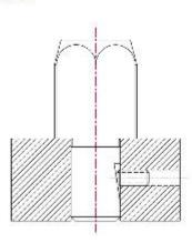
The Notch feature works the same way as the flat, but while driving the set screw in, you push the back of the head against the mounting surface.
