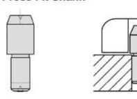
Shank is press fit into the base plate.
