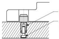
Shank is designed with slip fit tolerance
