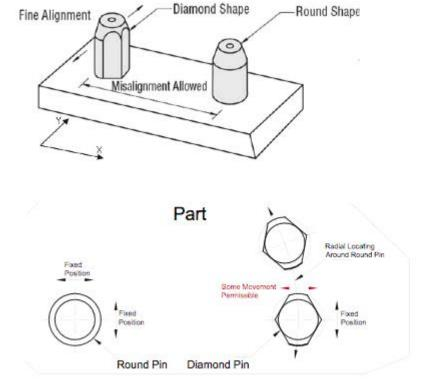
Please, see figure 2. The round pin is the datum pin that is located on the base and fixed in both X and Y direction. The Diamond pin oriented properly allows minimal misalignment in the X axis, but prevents the work piece to move in the Y direction. This way you eliminate small inaccuracies in respect to mounting hole distance and even if it's manufactured with high precision, the operation will improve since there is less work surface area.
