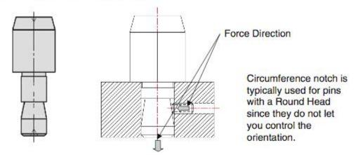
In some cases, there is no easy access on the back or the side of the pin mounting plate. There are a couple of standard solutions.
