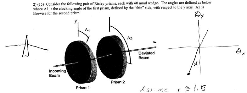
We wish use the prisms to make a linear scan of a laser beam in the y direction.
