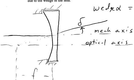
wedged =  $\frac{25\mu m}{25mm} = 1 \, \text{mrad}$ mech axis
