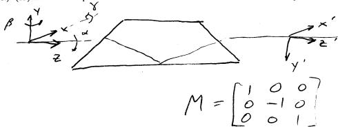
Define roll, pitch and yaw on your sketch. Provide the approximate change of line of sight and image rotation for small angular motions about each axis:
