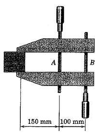
3) (5) Calculate the reactions at B for static equilibrium when a 10 lb vertical force is applied at A.
