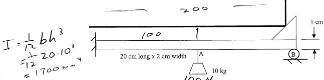
Use superposition to determine the change in pointing angle for the reflected laser beam when a 10 kg weight is attached at the middle of the beam.
