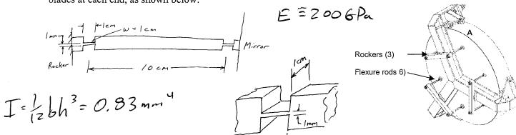
A) Calculate the angular stiffness for each 1 mm thick blade in the soft direction (in N-mm/mrad).
