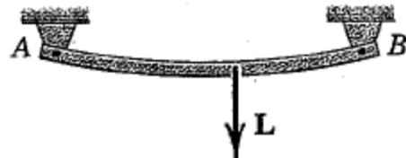
3. Loaded truss supported by pin joint at  $A$  and by cable at  $B$ .
