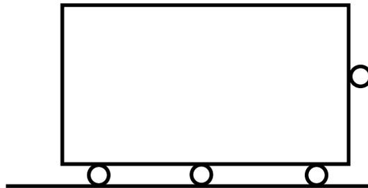
**A body that is neither overconstrained nor underconstrained is called static determinant**
