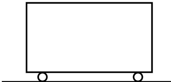
**If the mechanical constraints provide an attachment so that there is no unique solution for the reaction forces, the body is overconstrained**
