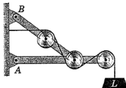
For a rigid body to be static, the net sum of forces and moments acting on it must be zero.
