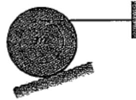
2. Wheel of mass  $m$  on verge of being rolled over curb by pull  $P$ .
