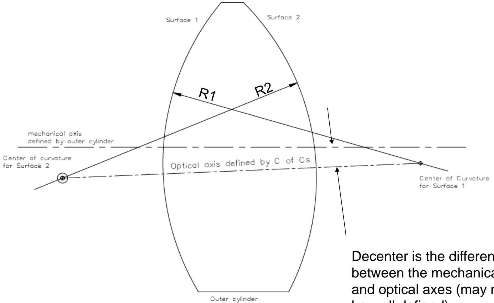
Decenter is the difference between the mechanical and optical axes (may not be well defined)
