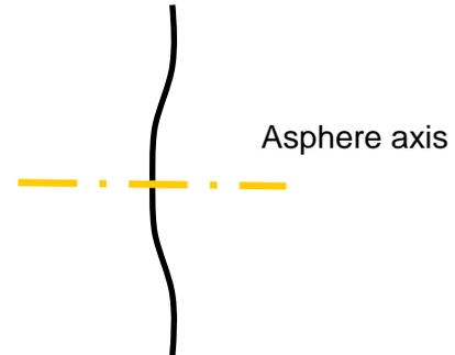
Lens with aspheric surface
