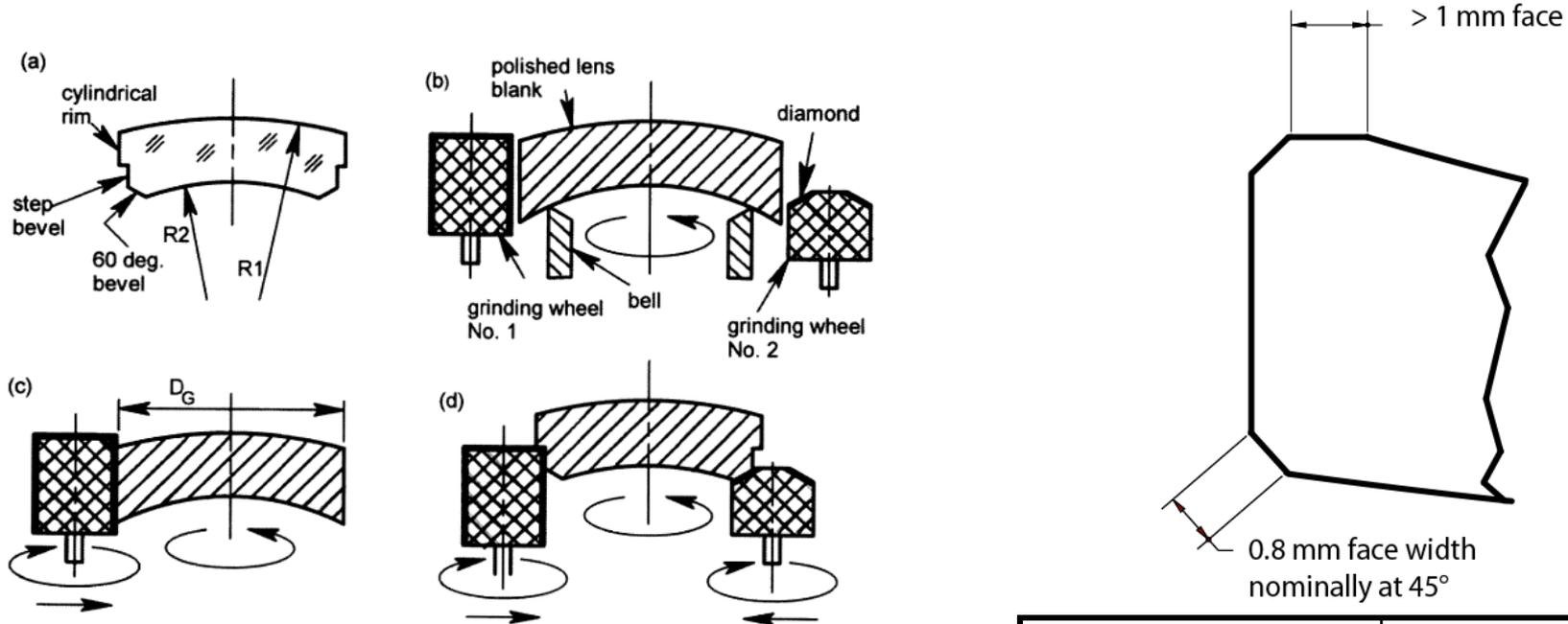
Figure 2.11 Producing various mechanical surfaces in addition to the rim on a lens element during edging.
