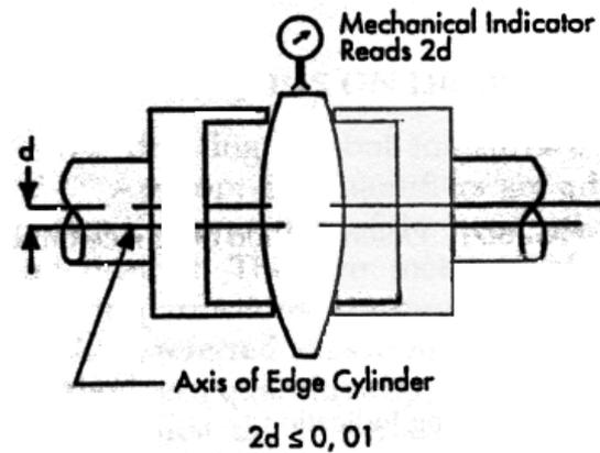
FIG. 6.5. Measurement of run-out of edge cylinder.
