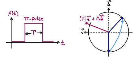
Idea is to measure population of  $|2\rangle$  as function of  $\Delta = \omega_{\gamma} - \omega$ , which is maximized for  $\omega = \omega_{\gamma}$ .
