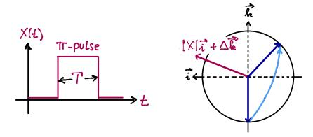
Idea is to measure population of  $\{2\}$  as function of  $\Delta = \omega_{\chi} - \omega$ , which is maximized for  $\omega = \omega_{\chi}$ .
