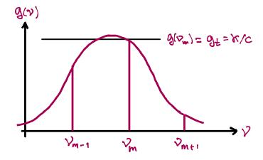
1st mode to reach threshold will lase, saturate gain, and clamp the inversion at its threshold value
