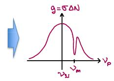
The pump saturates the gain for atoms with transition freq. near → only □
