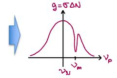
The pump saturates the gain for atoms with transition freq. near  $\searrow_m$  only
