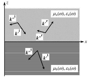
**Problem 2**) Inside a transparent dielectric prism of refractive index *n*, A monochromatic planewave of frequency  $\omega$  propagates along the *k*-vector  $\mathbf{k}^i = k_x \hat{\mathbf{x}} + k_z^i \hat{\mathbf{z}}$ , as shown. The plane-wave is linearly polarized along the *y*-axis (i.e., *s*-polarization). The incidence angle  $\theta^i$  is greater than the critical angle  $\theta_c = \sin^{-1}(1/n)$  of total internal reflection.
