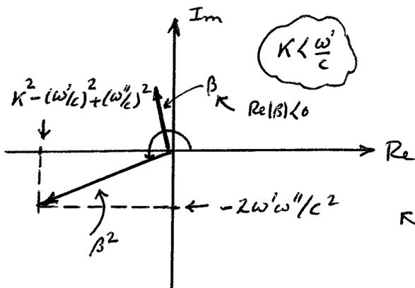
In the case of  $K < \omega'/c$ , we have  $\beta^2 = |\beta|^2 e^{i\phi}$  with  $\phi > 180^\circ$ . The  $\beta$  shown in the figure has a negative real part, thus the correct choice for  $\beta$  will be  $-i\sqrt{(\omega'/c)^2 - K^2}$ .
