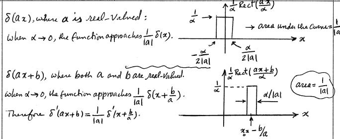
$$F\{\delta(x)\} = \lim_{\alpha \to 0} F\{\frac{1}{\alpha} \operatorname{Rect}(\frac{x}{\alpha})\} = \lim_{\alpha \to 0} \{\frac{1}{\alpha} \int_{-ikx}^{\alpha/2} dx\} = \lim_{\alpha \to 0} \frac{e^{-ik\alpha/2} + ik\alpha/2}{-i\alpha k}$$
