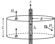
because of symmetry; its contribution to the surface integral will thus be  $2\pi RLH_{\rho}$ . The total integral of the *H*-field over the surface of the can is, therefore,  $2\pi RLH_{\rho}$ , which must be zero in accordance with Maxwell's 4<sup>th</sup> equation. We conclude that  $H_{\rho}(\rho, \phi, z)$  must be zero everywhere.
