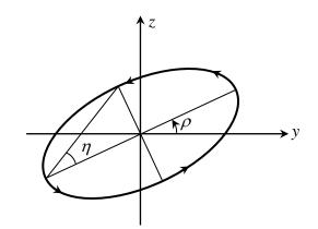
The above figure shows the ellipse of polarization oriented in the yz-plane in such a way that its major axis makes an angle  $\rho$  with the y-axis. The ellipticity of the state of polarization is denoted by  $\eta$ . The magnitude of the *E*-field along the major axis may thus be written as follows:
