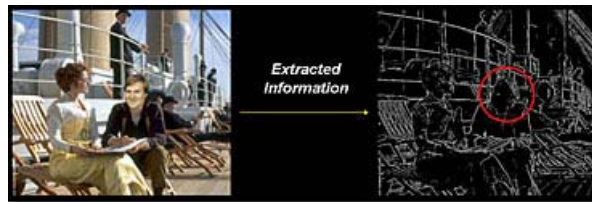
Figure 21: An image has an encoded watermark that contains the edge information of original image, revealing an alteration that has been made to the original image.
