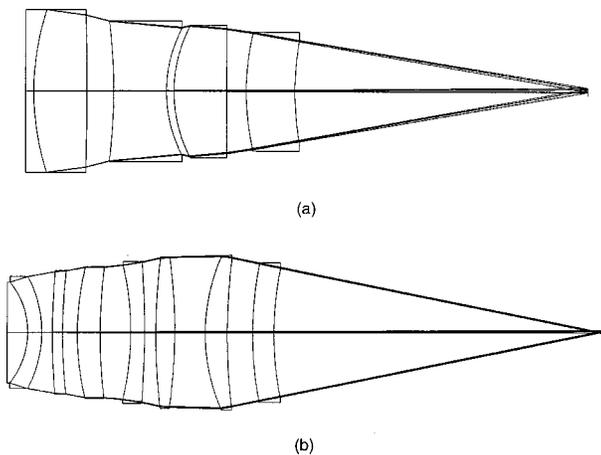
**Fig. 2** (a) The f/2.8 form shows a tendency in the lens design program to want fatter elements. In (b) the elements have been split and begin to show new forms such that the beam path encounters negative powers early on.
