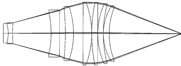
**Fig. 3** Fizeau transmission sphere operating at f/1.4 with a distance to focus of 375 mm.
