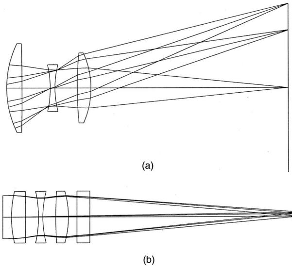
**Fig. 1** 50-mm f/5 Cooke triplet used as the starting point in the design (a) and modified (b) with reduced fields, monochromatic light, stop moved, and fused-silica plate added.
