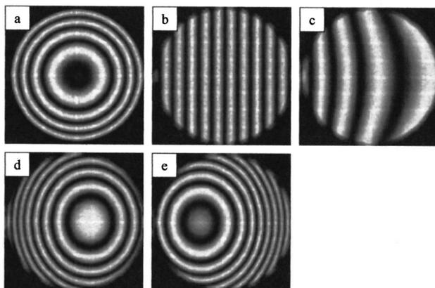
**Fig. 6** Interferograms obtained with the system of Fig. 5 when the test item is an aberration-free, spherical, uncoated glass mirror having  $R_c = -625$  mm. The fringe patterns shown are obtained with (a)  $20\text{-}\mu\text{m}$  of defocus, (b)  $50\text{-}\mu\text{m}$  of lateral shift, (c)  $0.1$  deg of tilt, (d)  $20\text{-}\mu\text{m}$  of defocus plus  $0.1$  deg of tilt, (e)  $20\text{-}\mu\text{m}$  of defocus,  $0.1$  deg of tilt, and  $50\text{-}\mu\text{m}$  of lateral shift.
