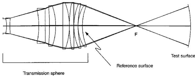
**Fig. 5** A seven-element  $f/1.4$  transmission sphere consisting of six elements of LaF2 and one element, containing the reference surface, of fused silica. The distance to the surface under test is twice the front focal length, which is 375 mm.
