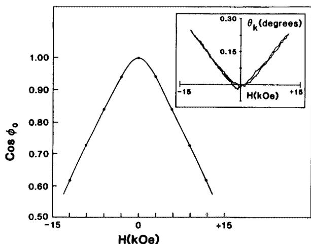
FIG. 3. Inset: Kerr rotation vs external in-plane field  $H$  for a  $\text{Tb}_{18.2}(\text{Fe}_{80}\text{Co}_{20})_{69.7}\text{Ar}_{12}$  sample. The main figure is the matching of the theoretical curve with the normalized  $(\theta_k/\theta_0)$  experimental data with  $\alpha = 3550$  and  $\beta = 3250$ .
