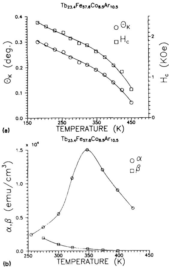
FIG. 6. (a) Kerr rotation ( $\theta_k$ ) and coercivity ( $H_c$ ) vs temperature. (b)  $\alpha$  and  $\beta$  vs temperature.
