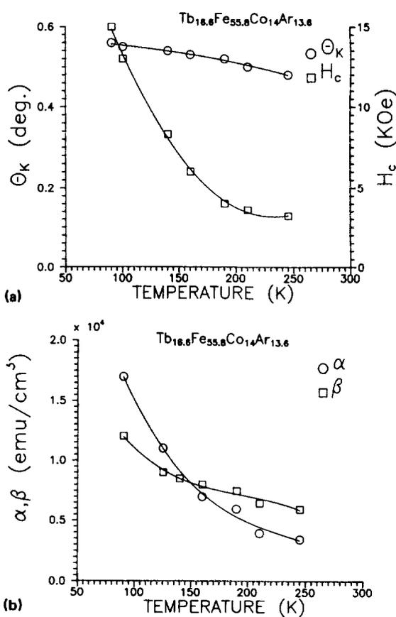
FIG. 5. (a) Kerr rotation ( $\theta_k$ ) and coercivity ( $H_c$ ) vs temperature. (b)  $\alpha$  and  $\beta$  vs temperature.
