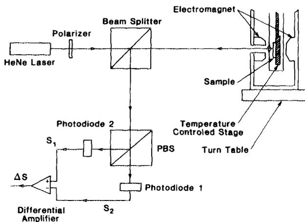
FIG. 1. Diagram of the measurement system.
