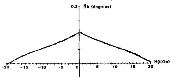
FIG. 7. In-plane measurement for a  $\text{Tb}_{21}\text{Fe}_{70}\text{Co}_9$  that cannot be fitted with the model.
