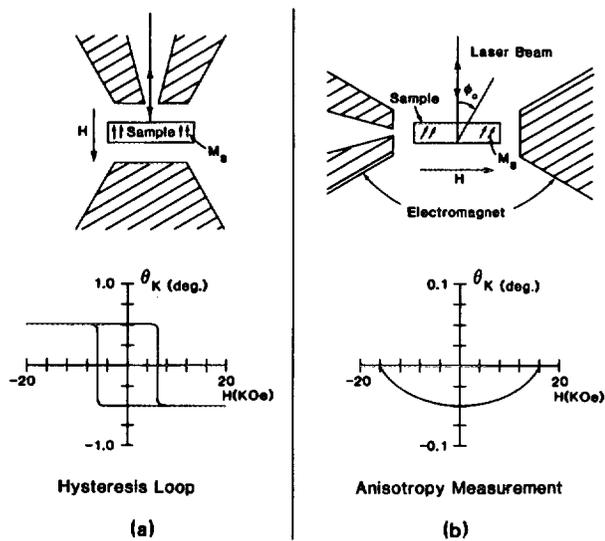
FIG. 2. Perpendicular (a) and in-plane (b) polar Kerr effect measurement.
