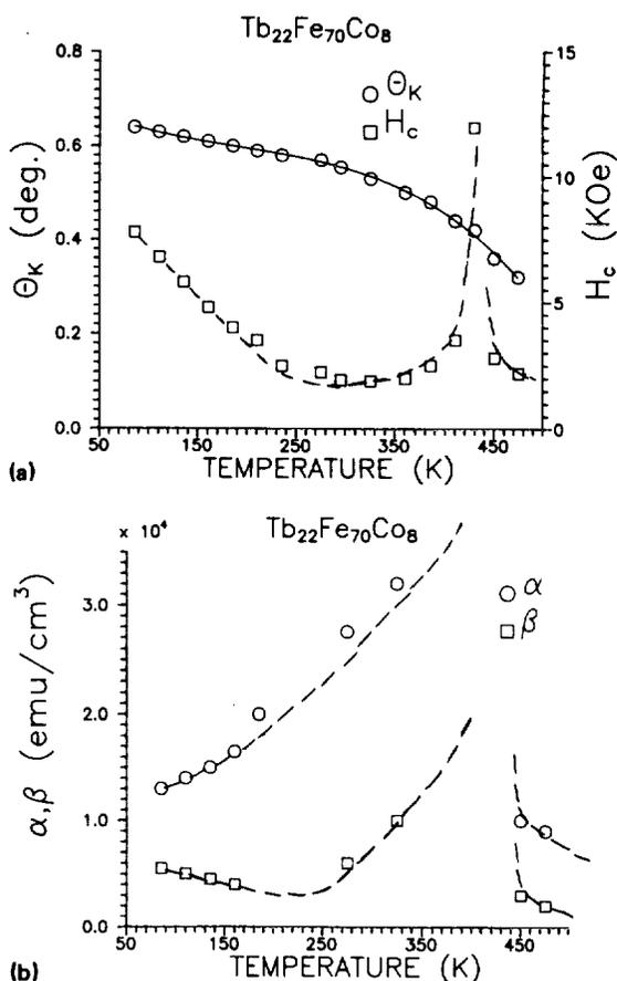
FIG. 4. (a) Kerr rotation ( $\theta_k$ ) and coercivity ( $H_c$ ) vs temperature. (b)  $\alpha$  and  $\beta$  vs temperature.
