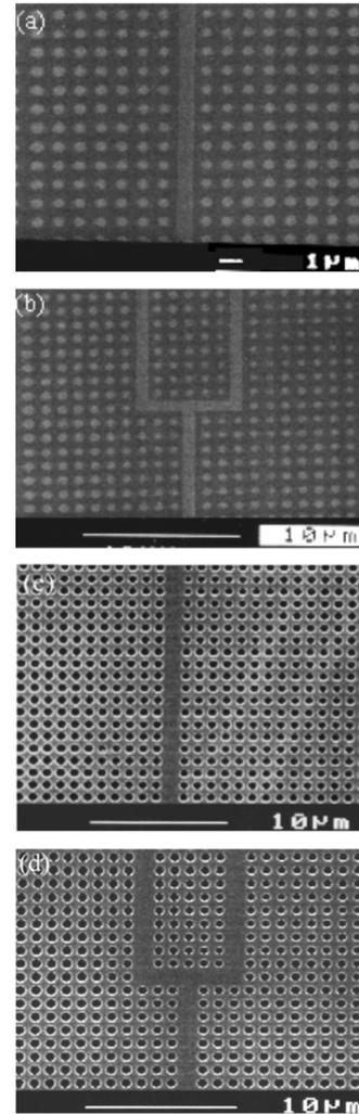
Fig. 3. (a) and (b) SEM micrographs of the PCs with defects in Cr. These figures correspond to Fig. 2(7). The  $\text{SiO}_2$  layer in the defect regions is clearly visible. (c) and (d) SEM micrographs of the PCs with defects in InP after removal of residual Cr. These figures correspond to Fig. 2(8).
