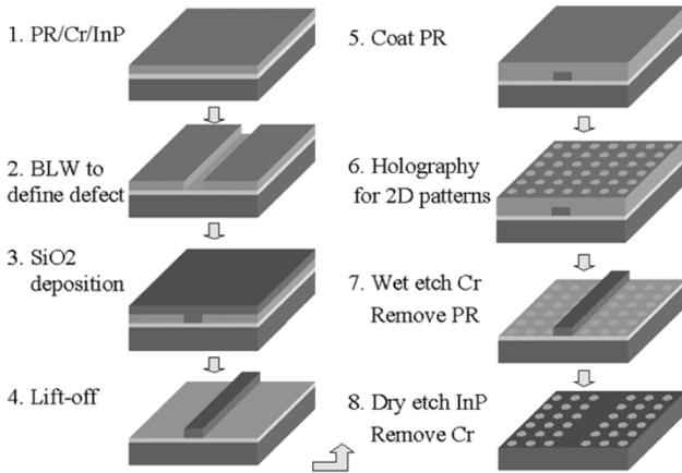
Fig. 2. Schematic of the fabrication procedures. PR: photoresist. BLW: blue-laser-writer.
