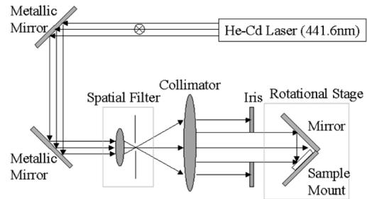
Fig. 1. Schematic of the two-beam interferometric optical holography. Objective lens in the spatial filter:  $X60/0.85$ . Pinhole in the spatial filter:  $5\ \mu\text{m}$ . Collimator:  $F5/250\ \text{mm}$ .
