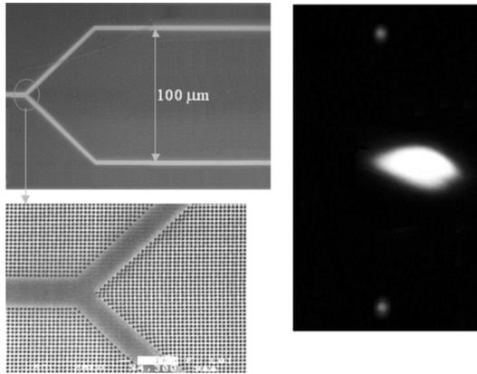
Fig. 4. Beam splitting at  $\lambda = 1540$  nm for TE polarization. Top: picture of the fabricated beam splitter (taken with an optical microscope). Bottom: SEM micrograph of the splitter region. Right: signals detected by an IR camera placed at the output end of the splitter for in-plane view. The total length of the structure is  $\sim 200$   $\mu\text{m}$ .
