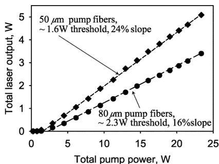
Fig. 4. Total power output of the laser at around 1535 nm, versus total pump power, for two different pump delivery fiber sizes. The data is shown with symbols, the linear fits with lines.
