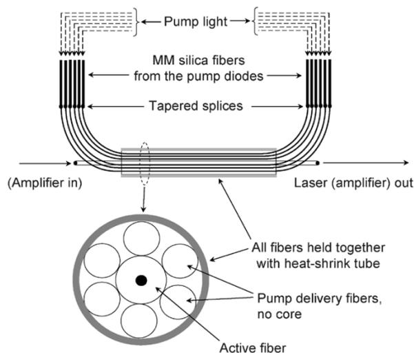
Fig. 1. Schematic diagram of the contact side-pumping scheme. The lower figure shows the cross section of the assembly.
