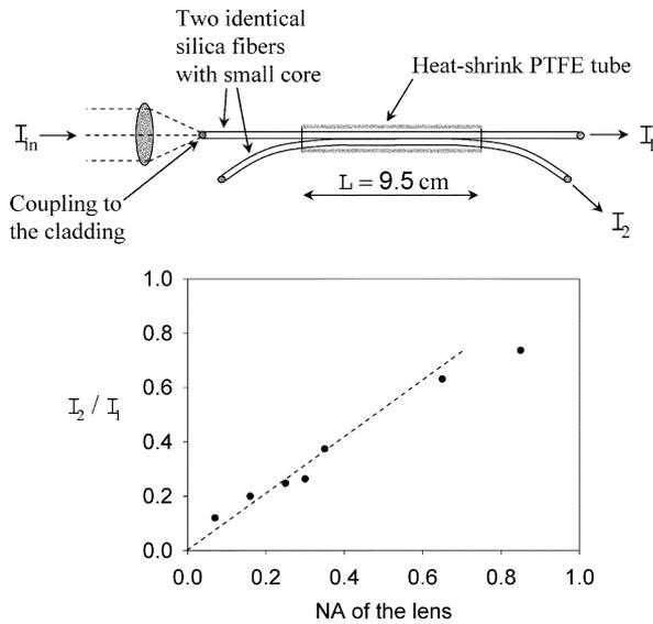
Fig. 2. Setup for measuring the dependence of evanescent coupling strength on the modal content of the propagating lightwave. The lower figure shows the measured ratio of the two outputs from the fibers as the NA of the coupling lens is varied.
