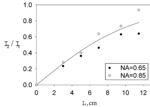
Fig. 3. Dependence of the coupling strength on the interaction length for two different NA values of the pump light source. The data is fit  $I_2/I_1 = \tanh(L/L_0)$ , with  $L_0 = 11 \text{ cm}$  (solid line). The measurement setup is the same as that in Fig. 2.
