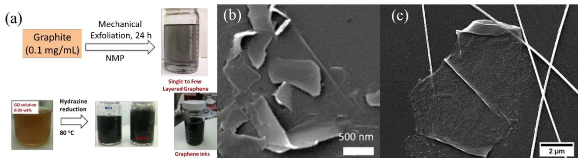
**Figure 5.** (a) Diagram showing liquid exfoliation for pristine graphene and reduction process for graphene oxide. (b) SEM image of graphene flakes deposited on a glass substrate. (c) SEM image of graphene flake with silver nanowires in a hybrid film.
