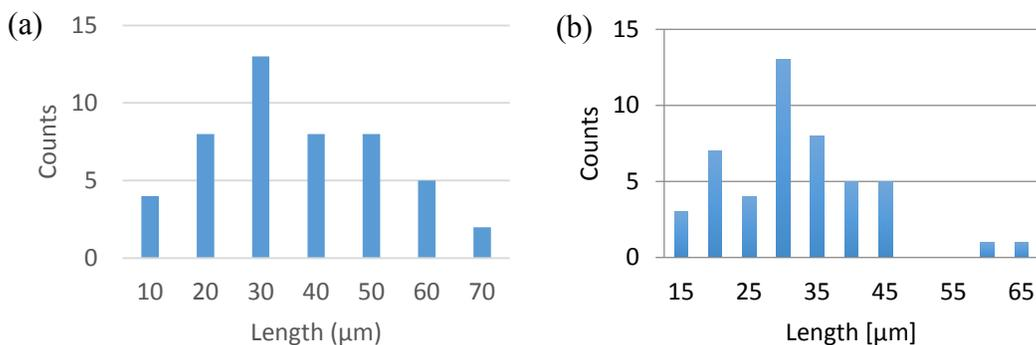
**Figure 2.** (a) Histogram of synthesized copper nanowire lengths. (b) Histogram of synthesized silver nanowire lengths. Both histograms were obtained from approximately fifty randomly selected nanowires.
