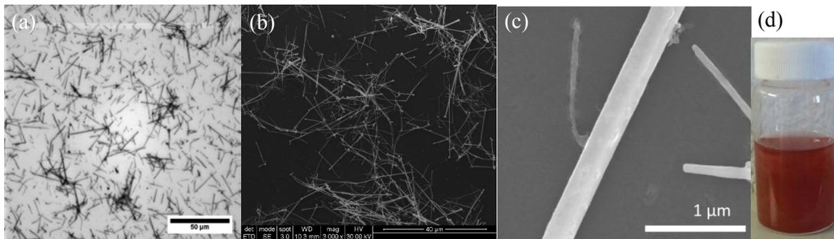
**Figure 1.** (a) Optical image of the synthesized copper nanowires. (b) SEM image. (c) Close-up SEM image showing wire diameters. (d) Homogeneous suspension of synthesized copper nanowires in a glass vial.
