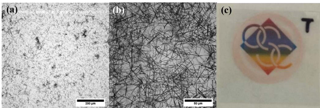
**Figure 3.** (a) Optical microscope image of spin-coated copper nanowire film. (b) Optical image of copper-nanowire film fabricated by vacuum filtration followed by transfer to a glass substrate. (c) Copper nanowire film fabricated by vacuum filtration followed by transfer to a plastic substrate (optical transmittance ~65%).
