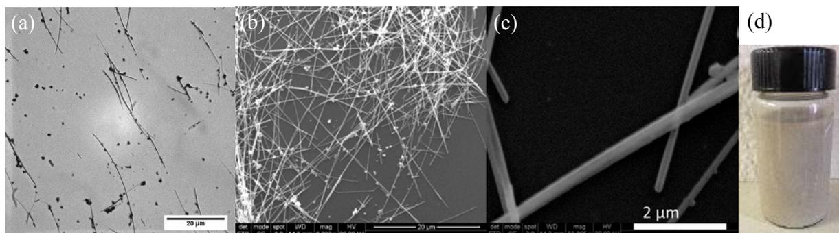
**Figure 4.** (a) Optical image of the synthesized silver nanowires. (b) SEM image of synthesized silver nanowires. (c) SEM image showing silver nanowire junctions. (d) Homogeneous suspension of synthesized silver nanowires in a vial.
