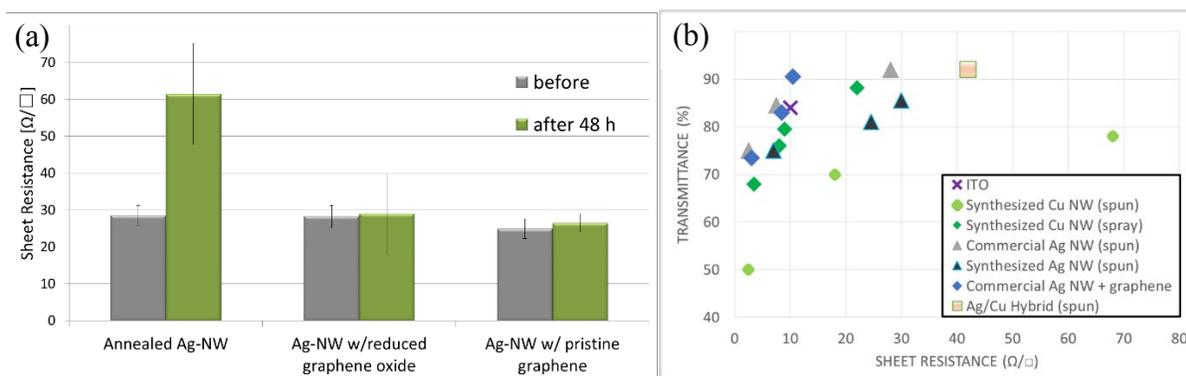
**Figure 6.** (a) Sheet resistance before and after harsh treatment at 80 °C and 80% relative humidity for silver and silver hybrid films. (b) Transmittance vs. sheet resistance for all reported materials and experimental methods in this work; also shown for comparison are the characteristics of conventional ITO transparent conductive electrode (×).
