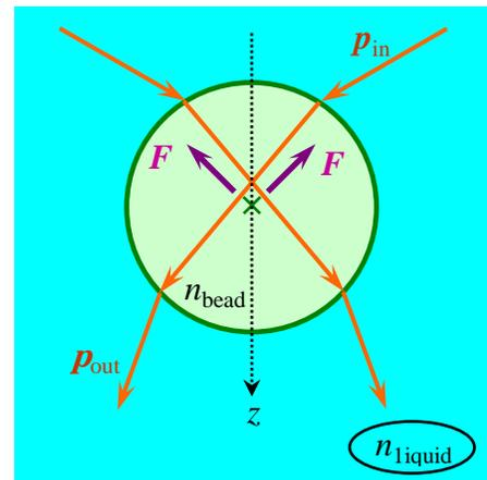
Fig.4. Single-beam optical trap.
