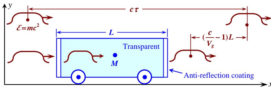
**Fig.7.** The thought experiment of Balazs involves the propagation of a light pulse of energy  $\mathcal{E}$  through a transparent rod of length  $L$  and mass  $M$ . The rod can move on a frictionless rail along the  $x$ -axis. Since the group velocity  $V_g = c/n_g$  of the pulse inside the rod is less than  $c$ , the emergent pulse is somewhat behind the location it would have reached had it travelled in vacuum all along.
