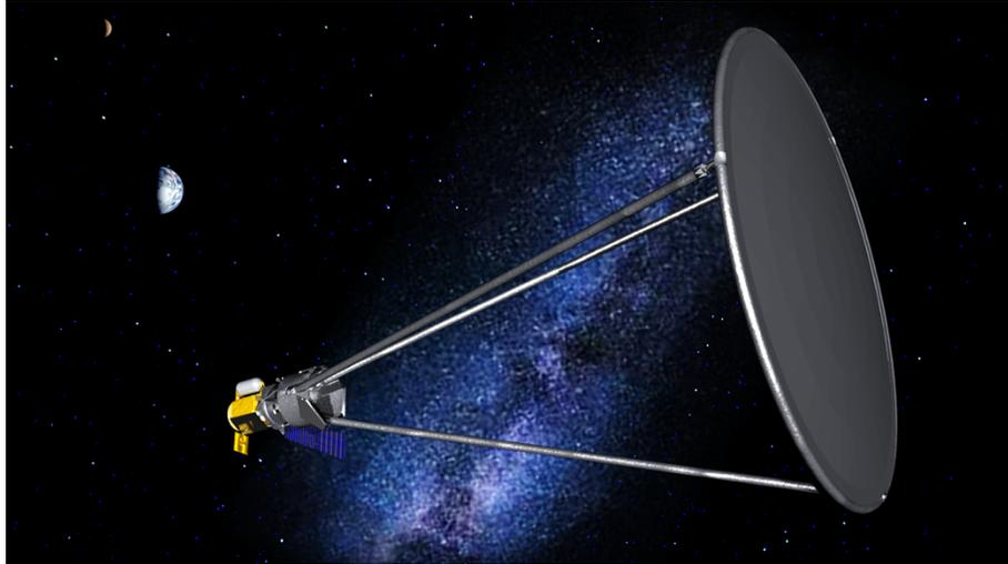
**Fig. 1.** OASIS Mission concept showing the 14 m diameter deployed inflatable membrane antenna (A1) configuration on the right side while the corrector optics and detectors are located inside the payload structure on the left.
