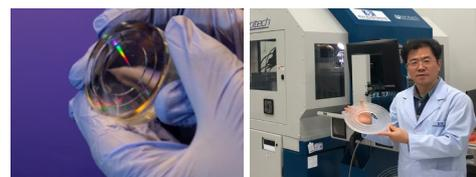
**Fig. 4.** MODE lens prototypes designed and fabricated with two diffractive surfaces of a front MODE surface and a single-order diffractive lens back-surface (left) [4] and a direct diamond turned 240 mm diameter MODE lens prototype (right).
