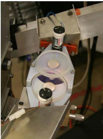
Fig. 17. SES made of two tilted spinning windows.
