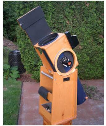
▲ **EVOLUTION OF THE 8-INCH** At left is the first version of my Newtonian on a Modified English Yoke Mount, while the right-hand photo shows the current incarnation, a fixed-height-eyepiece Dobsonian.
