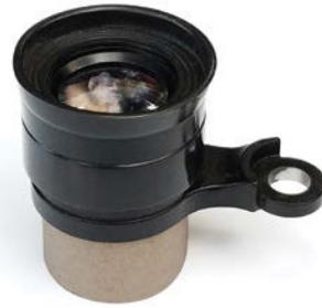
◀ **SCAVENGED OCULAR** A binocular eyepiece works just as well in a telescope as it does in binoculars.
