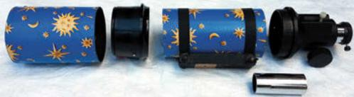
▲ The body tube slips inside the lens cell. The dew shield slides over the top. Note how much of the focuser's drawtube I had to cut off to avoid vignetting the steep light cone from the f/5 objective lens.
