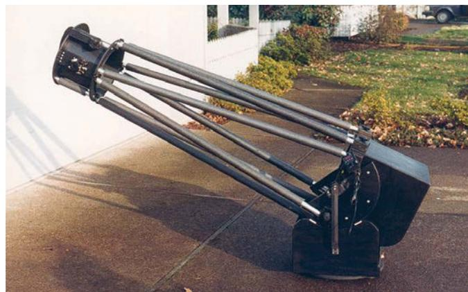
▲ **TINKERING AWAY** Above is the rebuilt 12.5-inch f/7.8 Dobsonian as it appeared after getting the 20-inch Obsession. The original was a basic but functional Dob built from bits and pieces of repurposed wood. It sported a long Sonotube optical tube painted green — which I apparently never photographed.
