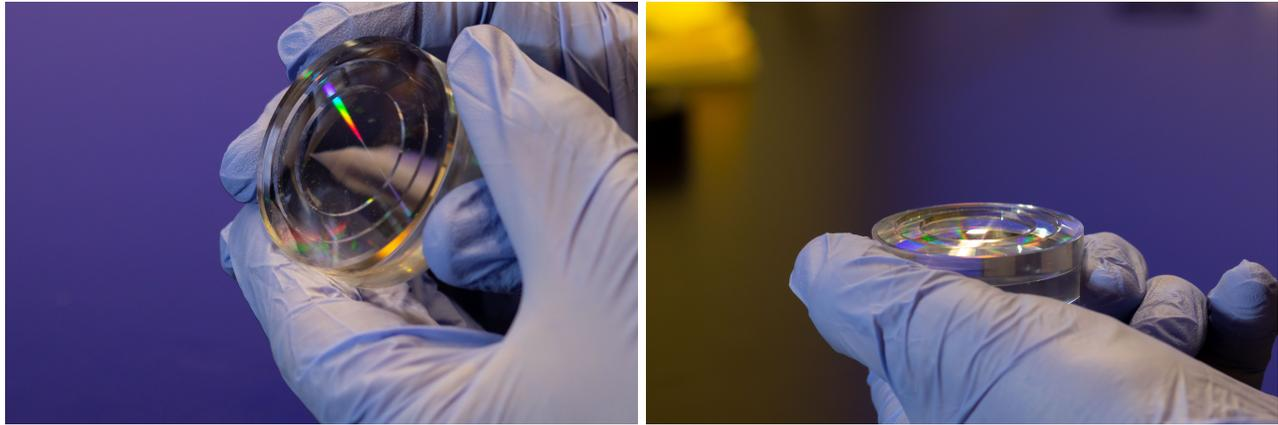
Figure 1. MODE lens prototype designed and fabricated by our University of Arizona team. This prototype has two diffractive surfaces (a front MODE surface and a traditional, single-order diffractive Fresnel lens backsurface). The combination of the two diffractive surfaces and the refractive component results in a very favorable chromatic performance.
