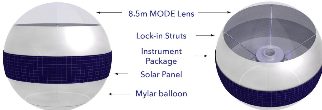
Figure 2. The Nautilus telescopes are launched in a compact configuration (b) and inflated in orbit (a). The inflation of the mylar balloon deploys the MODE lens (c). Due to the compact launch configuration, as many as 25 Nautilus units could be launched simultaneously in next-generation of fairings.
