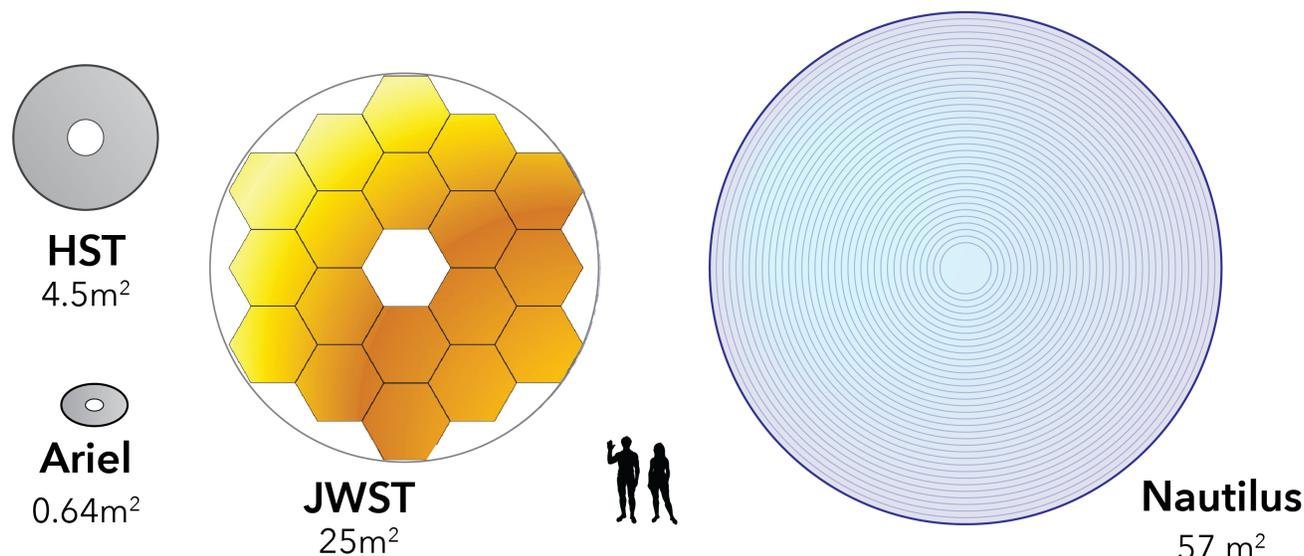
Figure 3. Comparison of the light-collecting area of space telescopes capable of exoplanet transmission spectroscopy. With its 8.5m diameter a Nautilus unit telescope's light-collecting area would exceed the combined light-collecting area of HST, Ariel (ESA's upcoming exoplanet characterization mission<sup>25</sup>), and JWST.
