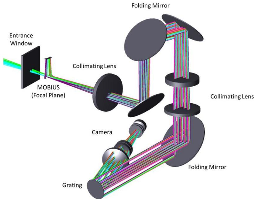
Figure 2. Optical layout shows MOBIUS introduced at the focal plane of LBT. By substituting the traditional slit frame mask with MOBIUS, LUCI is able to produce zJHK spectrum in a single exposure without any modifications in current instrument settings.
