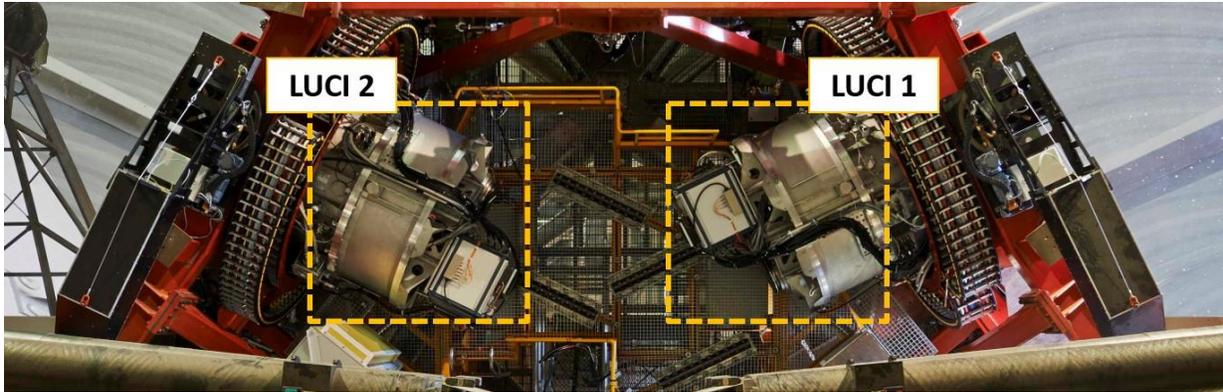
Figure 1. LUCIs on LBT.<sup>6</sup> LUCIs can have same (twinned mode) or different configurations (fraternal twin mode).<sup>4</sup> Also, at the binocular mode of LBT, each side could be configured with different instruments (mixed-mode) such as LUCI and MODS
