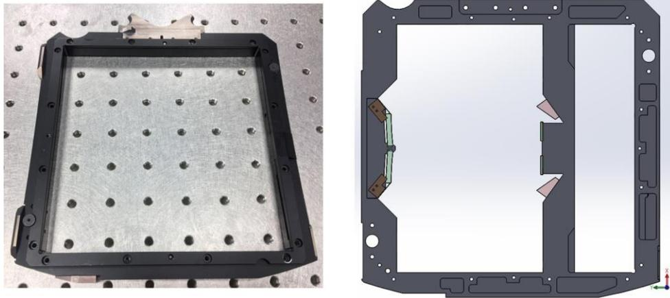
Figure 5. Slit frame of LUCI (left) and estimated 3D modelling of MOBIUS built in the frame (right). To compensate the additional weights of MOBIUS, light weighting features are included in the frame.
