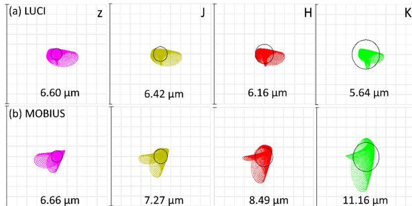
Figure 7. Spot diagrams at the focal plane of LBT when (a) LUCI only and (b) LUCI+MOBIUS is applied. The numbers in figure represent the rms spot radius of each spot diagram. Although the rms spot radius is slightly increased after the MOBIUS, it is still nearly the size of Airy's disk. Also, considering the smallest expected FWHM at the focal plane delivered from the telescope is  $150 \mu\text{m}$  or  $0.25$  arcsecond, the image quality is dominated by the atmospheric seeing.
