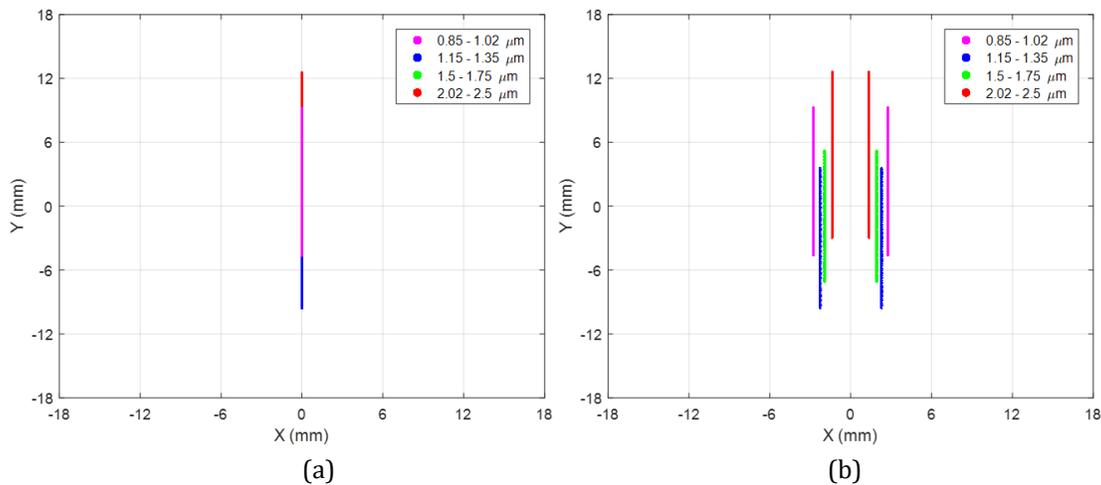
Figure 6. Footprint diagram at the detector when observing (a) only using LUCI and (b) LUCI with MOBIUS. With MOBIUS, spectra of each order are not overlapped. MOBIUS allows slit length up to  $\sim 2.3$  arcsecond.
