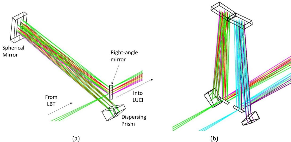
Figure 4. Optical layouts of MOBIUS. (a) shows an unit of MOBIUS. and (b) shows the overall layout of MOBIUS with two identical spectrograph units located side by side. For the sky subtraction by dithering, we flipped one unit to allow placement of the two entrance slits as close as possible.
