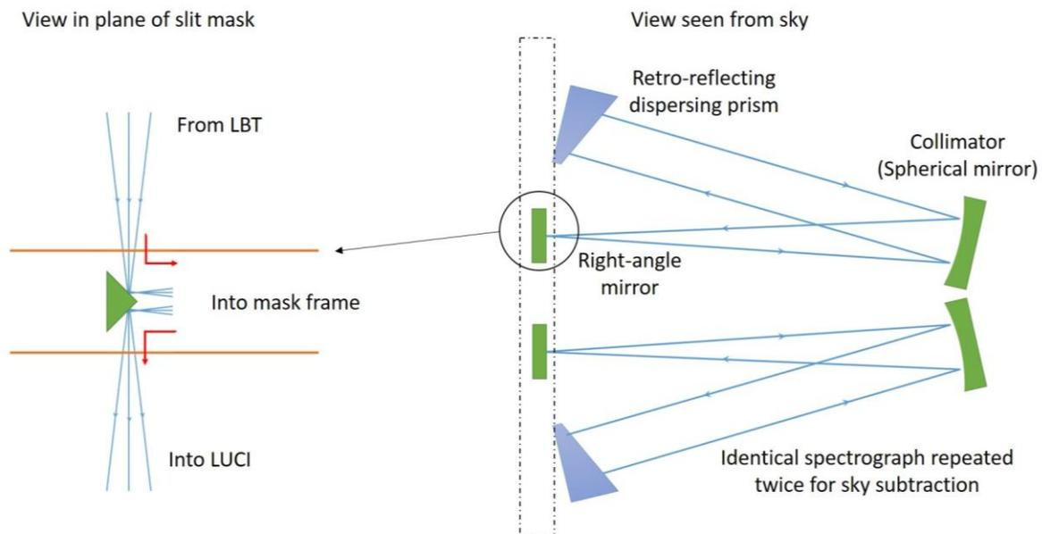
Figure 3. Schematic figure of MOBIUS a modular cross-disperser for LUCI. The right-angle mirror is inserted near the focal point of LBT to deflect the incoming beam from the LBT into the mask frame. Inside of the frame mask the beam is collimated and dispersed, then it is returned to the previous light path. Through this process, the input beam is cross dispersed before the higher dispersion grating in LUCI.
