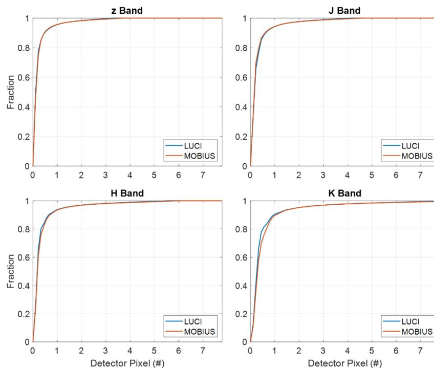
Figure 8. Ensquared energy comparison between LUCI and LUCI with MOBIUS. The difference in half width distance between LUCI and MOBIUS for 90% fraction energy is less than a pixel (on detector). Considering the seeing disk is  $>2$  pixels or  $0.25$  arcsecond, this difference is insignificant.
