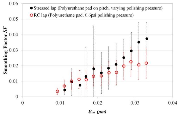
Figure 5. Smoothing efficiency comparison:  $SF$  vs.  $\epsilon_{ini}$  (initial local surface RMS error) for 800mm stressed lap with polyurethane pads on pitch tiles (black solid circle) and 250mm RC lap with polyurethane pad (red open circle). (The bar represents the spread (+/-  $1\sigma$ , standard deviation) of the  $SF$  values.)
