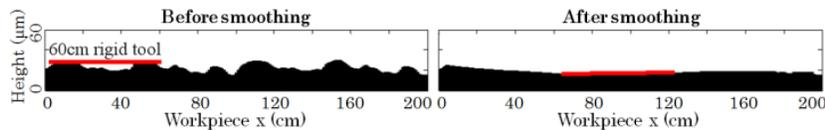
Figure 2. A schematic diagram showing the smoothing effect using an infinitely rigid tool [14]
