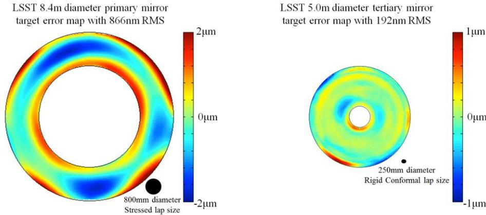
Figure 4. LSST primary (left) and tertiary (right) mirror surface error map before the CCOS runs, which were used as the target removal maps during the runs. The relative tool (contact area) size is depicted as a black disk in the bottom-corner.
