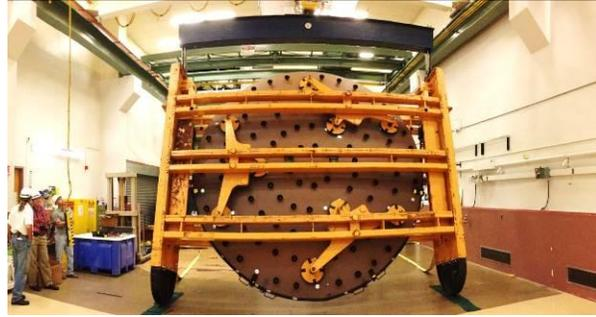
Figure 1. 4.2m diameter Advanced Technology Solar Telescope (ATST) off-axis primary Zerodur workpiece, which has a tight bidirectional reflectance distribution function (BRDF) specification to suppress the light scattering from the mirror surface, during the mirror flipping operation in the Optical Engineering and Fabrication Facility (OEFF) at the University of Arizona
