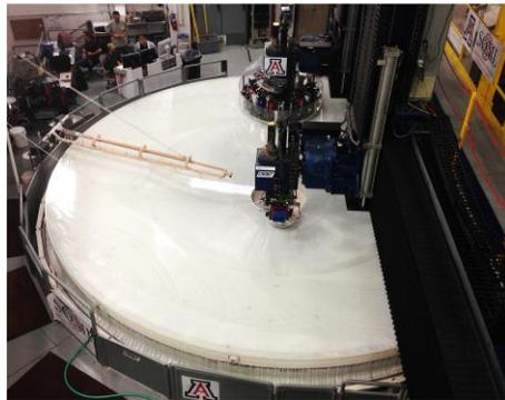
Figure 3. 8.4m diameter Large Synoptic Survey Telescope monolithic primary-tertiary mirror (primary on outside and tertiary on inside) under the large polishing machine equipped with the fraternal twin polishing tools, the stressed lap (top in the picture) and the RC (Rigid Conformal) lap (middle in the picture) in the Steward Observatory Mirror Laboratory at the University of Arizona.
