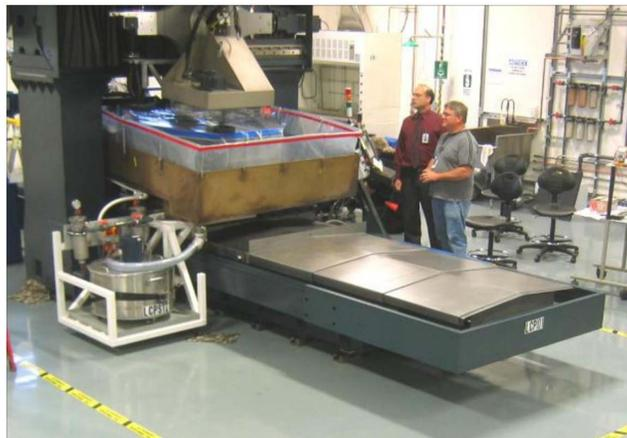
Aluminum surrogate of a JWST hexagonal segment during grinding tests at Tinsley on their computer-controlled optical surfacing machine. Image credit: J. C. Cole. Reprinted with permission from Cole *et al.*, Proc. SPIE **6265**, 62650V (2006) [120].
