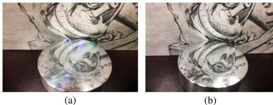
**Fig. 11** Visual appearance of the Al6061 sample (a) before and (b) after the smoothing process.
