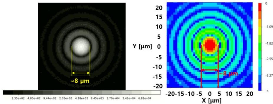
Fig. 3. Log scaled PSF simulation result of PhoSim (left) and CODE V (right).
