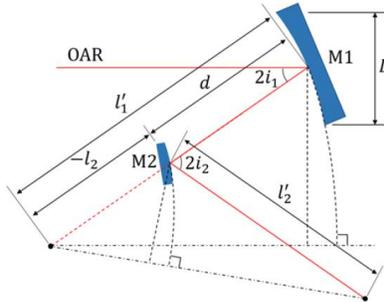
Fig. 2. Optical layout of the unobscured two-mirror confocal Cassegrain optical system.
