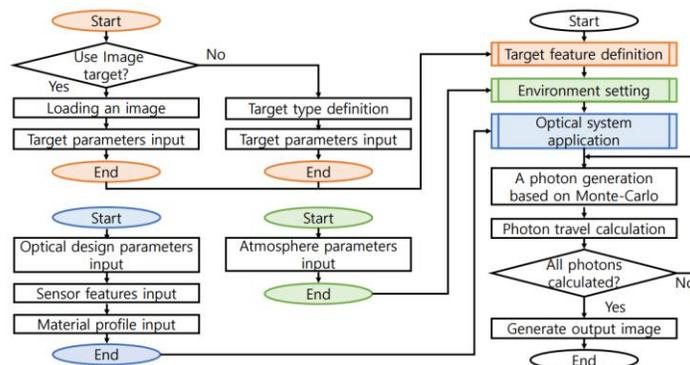
Fig. 1. Algorithm flowchart of PhoSim.
